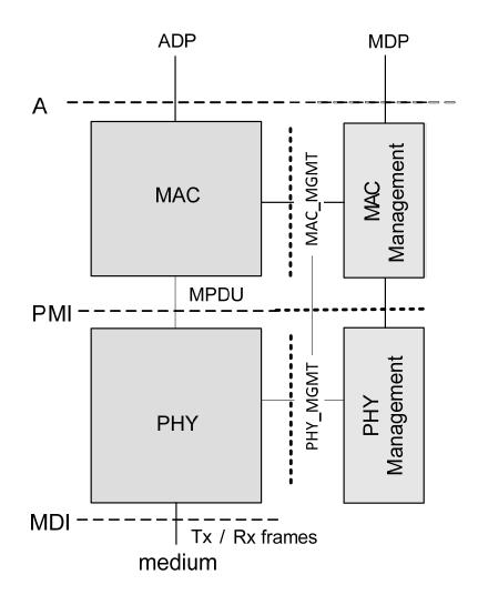
Figure 5-5 – Functional model of an ITU-T G.9959 transceiver
