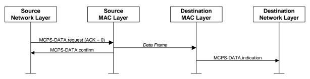
Figure 8-22 – Successful data transmission without an acknowledgment
