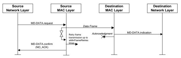
Figure 8-26 – Lost acknowledgment frame transmission scenario
