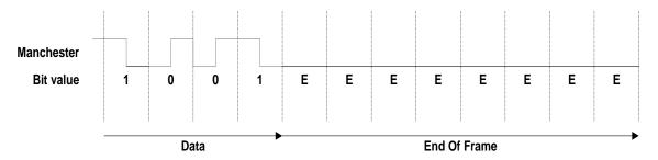
Figure A.10 – End of frame delimiter (EFD) pattern (R2/R3)
