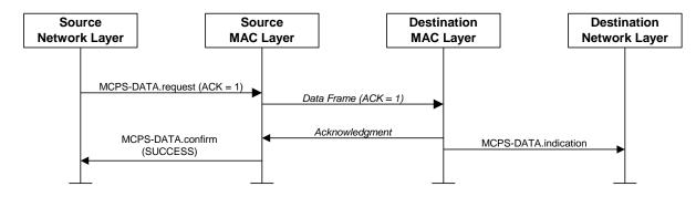
Figure A.34 – Lost frame transmission scenario
