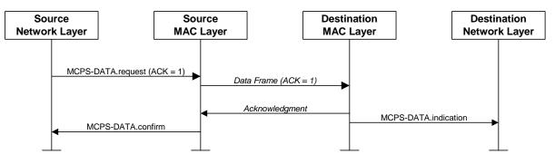
Figure 8-23 – Successful data transmission with an acknowledgment frame
