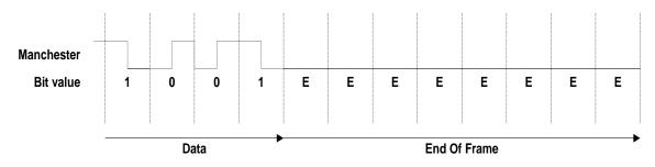
Figure 7-7 – End of frame delimiter pattern
