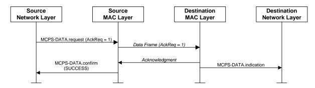
Figure A.33 – Successful frame transmission scenario
