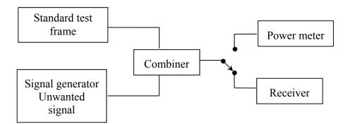
Figure A.6 – Receiver blocking test definitions
