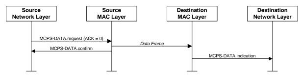
Figure A.31 – Successful data transmission without an acknowledgment
