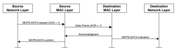
Figure A.32 – Successful data transmission with an acknowledgment frame
