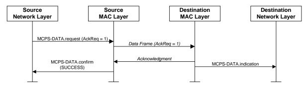
Figure 8-24 – Successful frame transmission scenario
