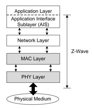
Figure A.2 – Z-Wave layers
