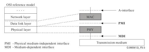
Figure 5-3 – Protocol reference model of an ITU-T G.9959 transceiver
