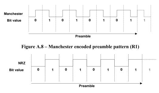
Figure A.9 – NRZ encoded preamble pattern (R2/R3)
