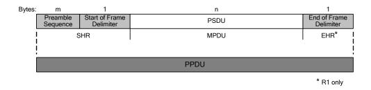
**Figure 7-4 – PPDU packet format**
