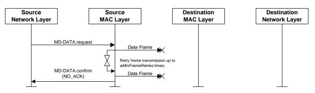
Figure 8-25 – Lost frame transmission scenario
