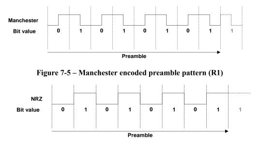
Figure 7-6 – NRZ encoded preamble pattern (R2/R3)
