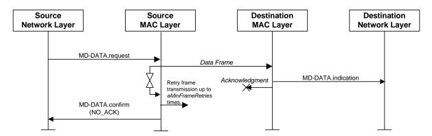
Figure A.35 – Lost acknowledgment frame transmission scenario
